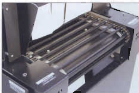
Standard Live Roller with 1" Roller Spacing
