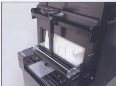
TPF System- Thin Package Fixture Keeps Package From Distorting in Tunnel
